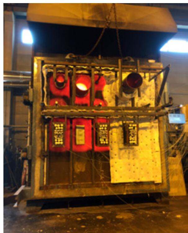
Foto: Firesafe AS Hydrokarbonbrann i skott.
